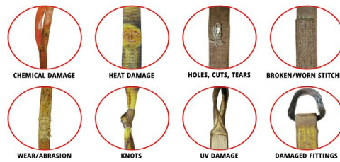
Nylon Rigging Hazards
